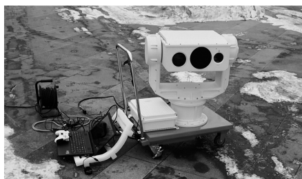
图 1 转台及高清可见光相机实物图 Fig.1 Picture of turntable and HD camera
