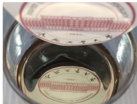
图 1 水油两相界面处的银纳米颗粒单层膜镜面反射效果 Fig.1 Mirror reflection effect of silver nanoparticles monolayer at the interface between water phase and oil phase
