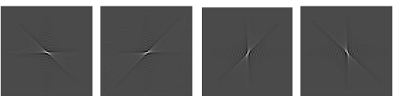
(f)第一层 4 个方向时域支撑的剪切滤波器 (f)Four direction time-domain implemented shear filters in the first level
