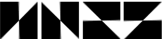
(e)第一层 4 个方向频域支撑的剪切滤波器 (e) Four direction frequency-domain implemented shear filters in the first level
