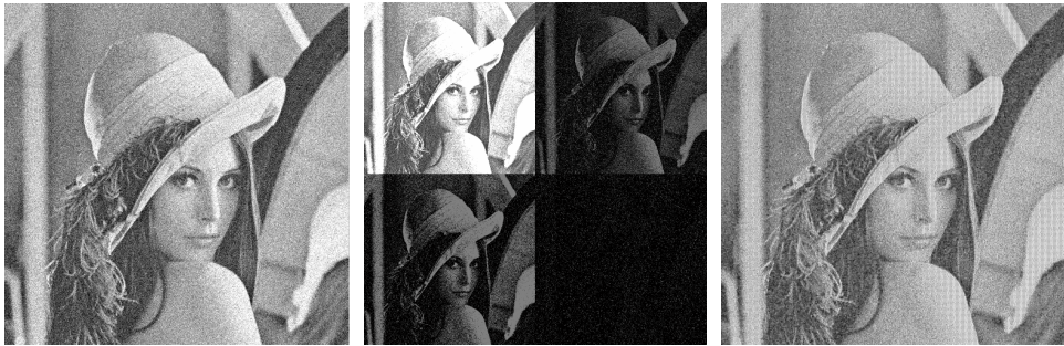
图 4 高斯噪声方差 \rho=0.1 时的 5/3 提升小波去噪仿真结果。(a)带噪图像;(b)提升小波图像;(c)处理后图像。 Fig. 4 Simulation results of 5/3 lifting wavelets when Gaussian noise Variance \rho=0.1 . (a)Image with Gaussian noise; (b) Image of 5/3 lifting wavelets;(c)Image after processing.
