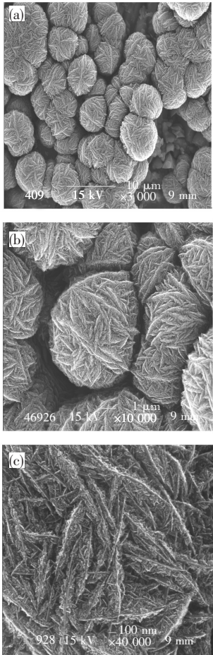
图 2 典型的碳纳米球薄膜 FESEM 图像. (b)和(c)为 (a)放大的图像. Fig. 2 SEM images of a typical carbon nanometer ball film. (b) and (c) are parts of magnified area of (a).
