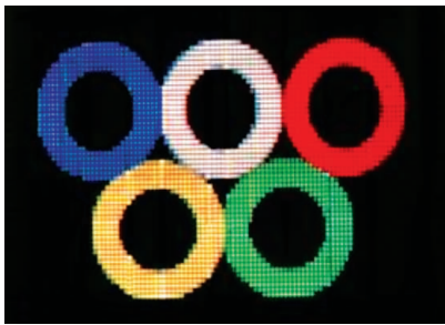
图 5 华南理工大学研制的 3.8 cm(1.5 in)无源 PLED Fig. 5 3.8 cm(1.5 in)PM-LED made by SCUT
