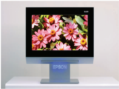
图 4 Epson 研制的 102 cm(40 in)1 280×768 LTPS TFT 驱动的 PLED Fig. 4 102 cm(40 in) PLED with LTPS TFT developed by Epson
