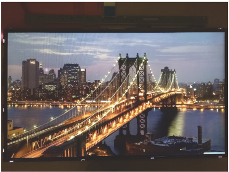
图 7 812 mm(28 in)色阻堆叠形成隔垫物显示屏 Fig.7 812 mm(28 in) display demo with color filter stacking as photo spacer technology
