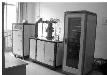
图 1 MPS-2050C 微波等离子化学气相沉积系统 Fig.1 MPS - 2050C microwave plasma chemical vapor deposition system
