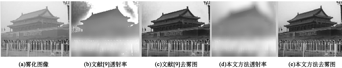
图 4 去雾效果及透射率分布对比(一) Fig.4 Comparison of Haze removal effect and transmittance distribution (1)
